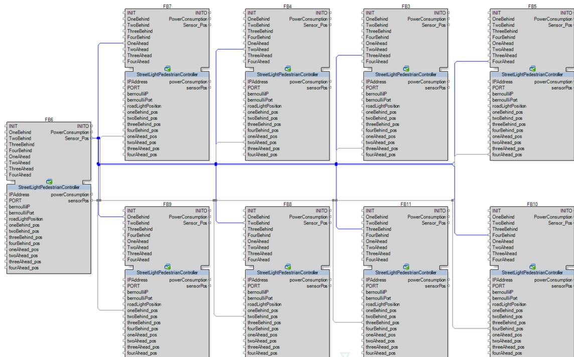
Fig. 1. An excerpt of a street light controller and its interconnections to four of its trailing and leading street light controllers
